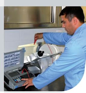
The MI 3310 SigmaGT is a multifunctional portable test instrument intended to perform all measurements for complete testing the electrical safety of portable electrical equipment. The instrument can operate from mains power or batteries.
